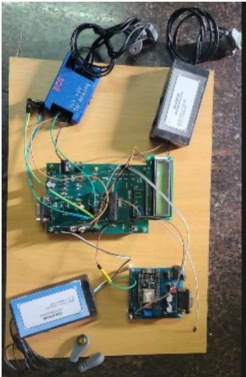
Fig. 2. Hardware setup of the proposed WBAN system including sensors, Arduino unit, NodeMCU module, and power supply
