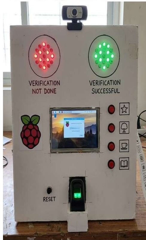
Fig. 7 Photograph of the assembled biometric voting system prototype showing the webcam for facial recognition, red (Verification Not Done) and green (Verification Successful) LED indicators, touchscreen display, ZA620 M5 fingerprint scanner, Reset button, and GPIO candidate selection buttons on the custom polling booth enclosure.
