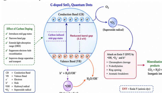
Figure 15. Proposed visible-light photocatalytic degradation mechanism of Eosin Y using C-doped SnO 2 quantum dots
