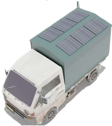
Fig. 35. Top view of the Mobile Health Care Dispensary with attached solar panels.
