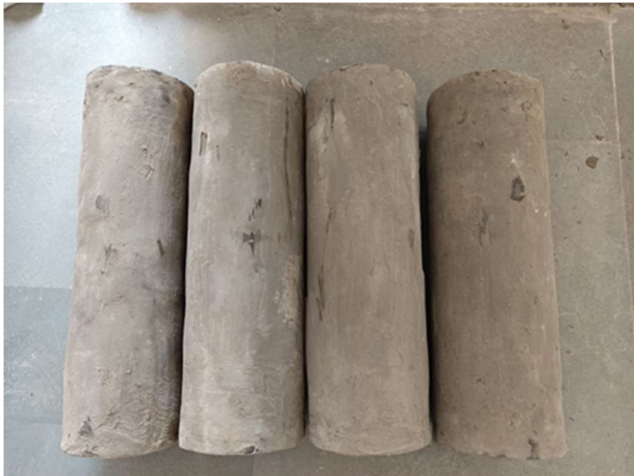
Fig. 2. Ferromesh unwrapped cement concrete-confined short concrete columns [control columns]
