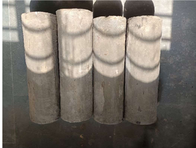
Fig. 7. Three layers of ferromesh-wrapped cement concrete-confined short concrete columns
