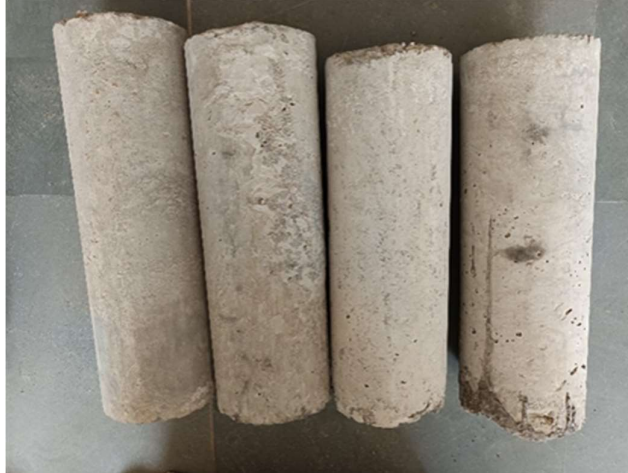
Fig. 4. One-layer ferromesh-wrapped geopolymer concrete-confined short concrete columns
