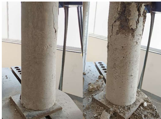
Fig. 20. Crack pattern and ultimate failure mode of ferromesh-wrapped short concrete columns confined with geopolymer concrete under axial loading
