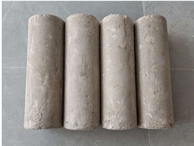
Fig. 5. Two layers of ferromesh-wrapped cement concrete-confined short concrete columns
