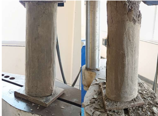
Fig. 19. Crack pattern and ultimate failure mode of ferromesh-wrapped short concrete columns confined with cement concrete under axial loading
