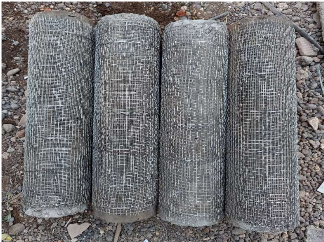
Fig. 1. Ferromesh wrapped short concrete columns
