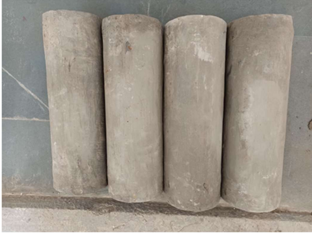
Fig. 3. One-layer ferromesh-wrapped cement concrete-confined short concrete columns
