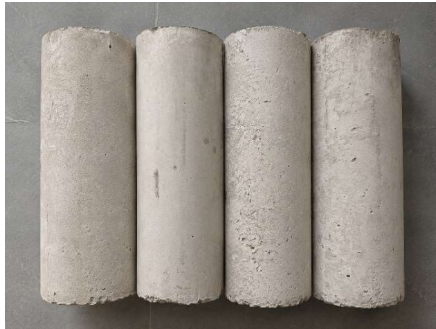
Fig. 8. Three layers of ferromesh wrapped geopolymer concrete-confined short concrete columns
