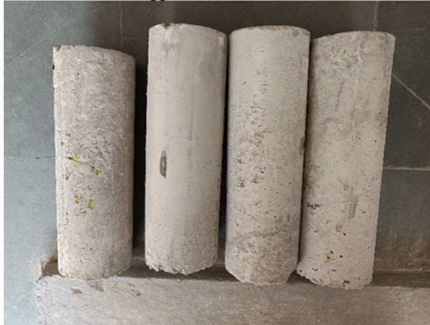
Fig. 6. Two layers of ferromesh-wrapped geopolymer concrete-confined short concrete columns
