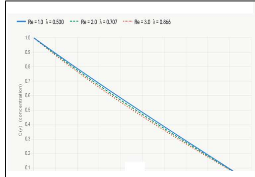
Figure 5: Concentration Profile for various values of Reynolds Number
