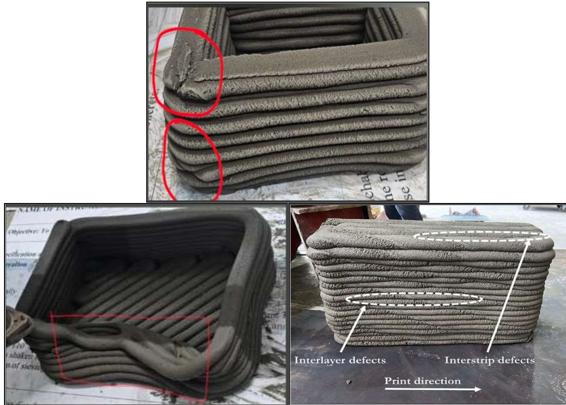
Fig 7: Defects in 3DPC
