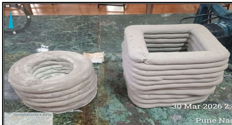
Fig 8: Hardened 3DPC circular and rectangular Models
