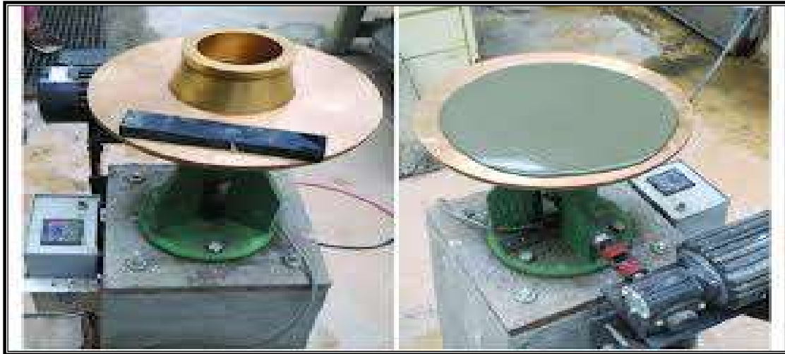
Fig 5: Flow test table as per ASTM-C1437
