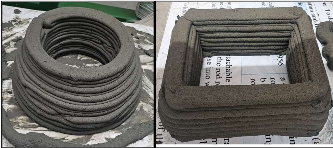
Fig 6: Freshly 3D printed circular and rectangular models
