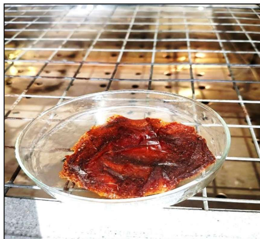
Fig. 5. Loss on drying test of the prepared film.
