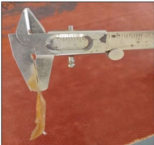
Fig. 2. Thickness measurement using Vernier calliper.
