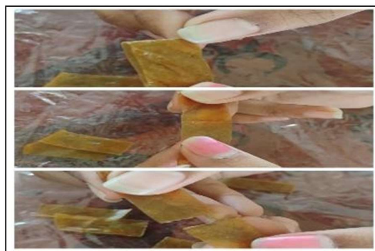
Fig. 4. Folding endurance test of the biodegradable film.
