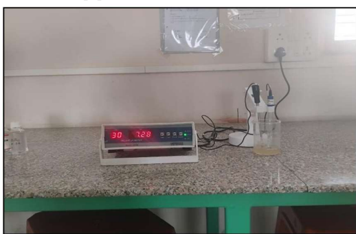
Fig. 3. pH test of the prepared film solution.
