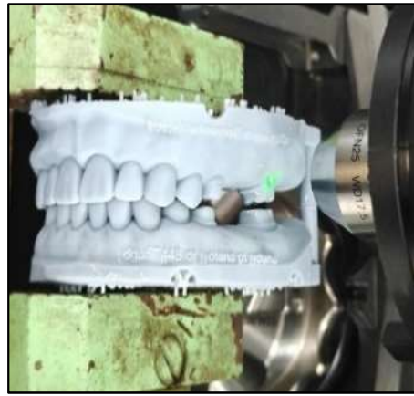
Fig 9: Measurement with Bruker Alicona uCMM Vision Inspection System.
