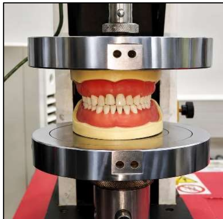
Fig 2: Force Application with UTM
