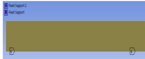
Figure 12: Fixed supports at span on reinforced concrete beam
