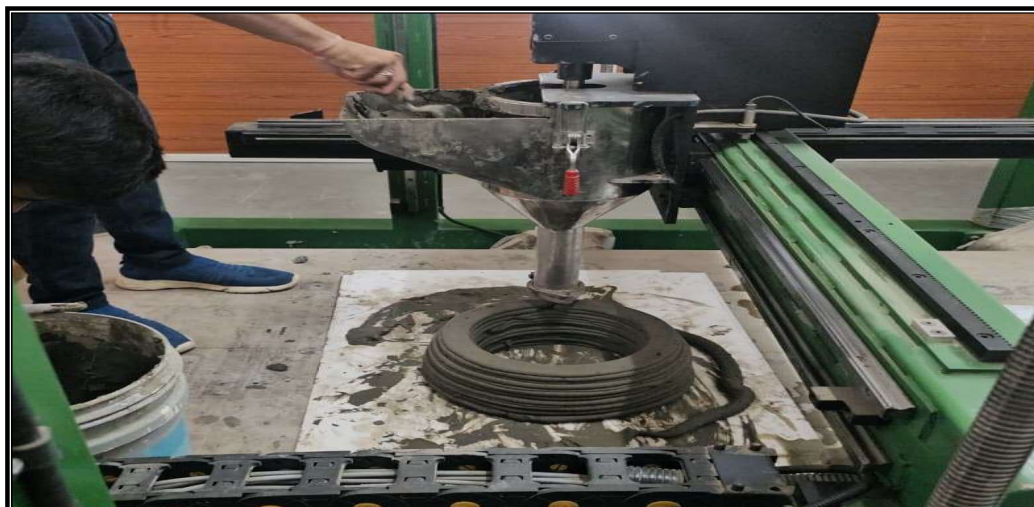
Fig 7: Extruding Process through 3DPC Gantry
