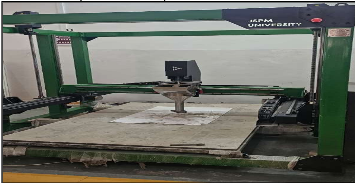
Fig 4: Deltasys E-Forming concrete 3D printer gantry (1m x 1m x 1m)
