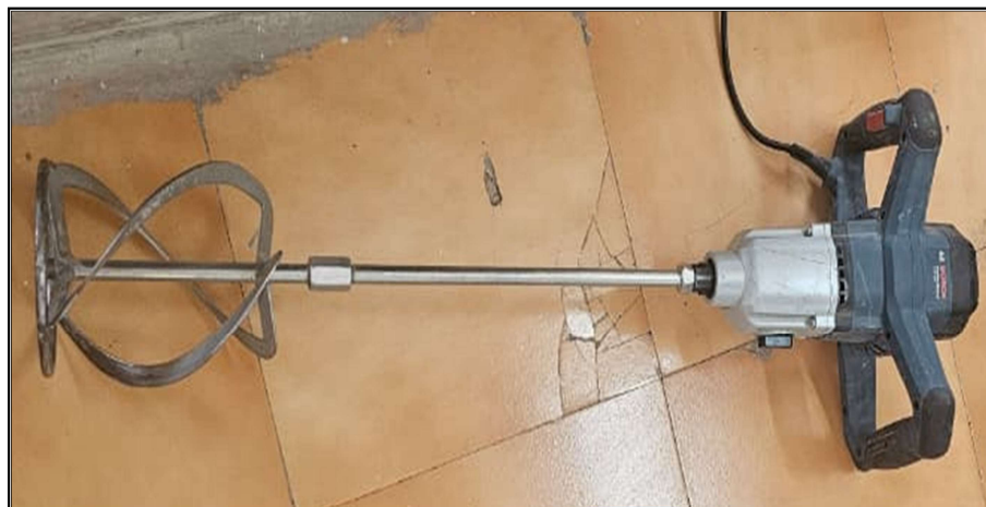
Fig 2: Bosch GBM 1600 RE Professional used for mixing concrete
