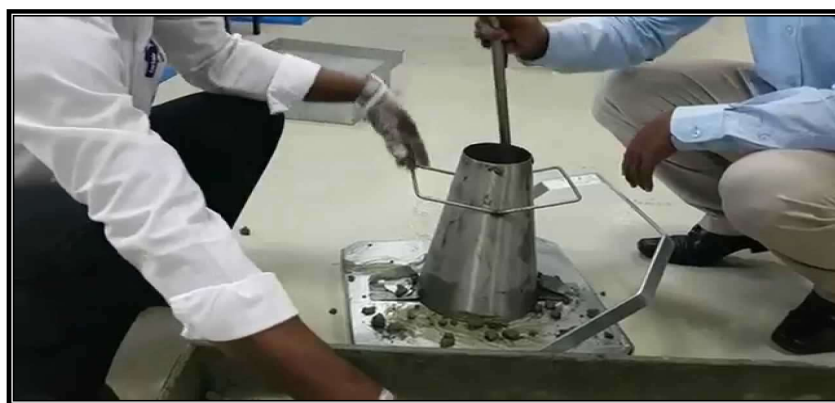
Fig. 6: Slump Cone test
