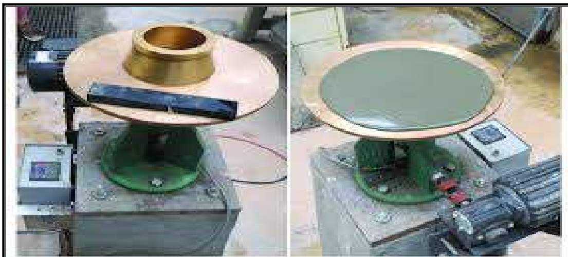
Fig 5: Flow test table as per ASTM-C1437
