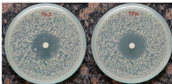
Figure 10: Zone of inhibition of optimized phloretin transethosome-loaded nail lacquer (NL2) and terbinafine (TFN) against Candida albicans by agar well diffusion method
