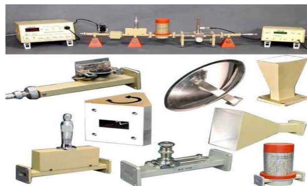
Fig. 3: X- Band Microwave Test Bench Setup
