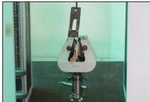
Figure Linear Load Applied Mediolaterally (double miniplate)
