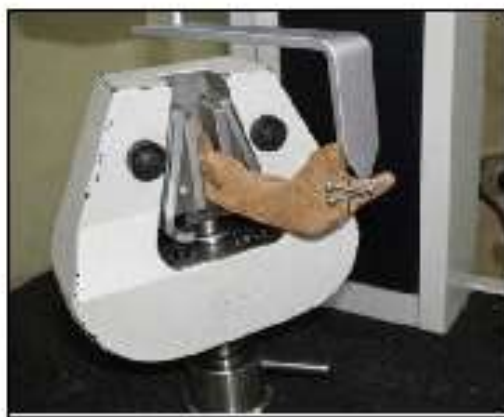
Figure Linear Load Applied In Anteroposterior Direction (Delta Plate)
