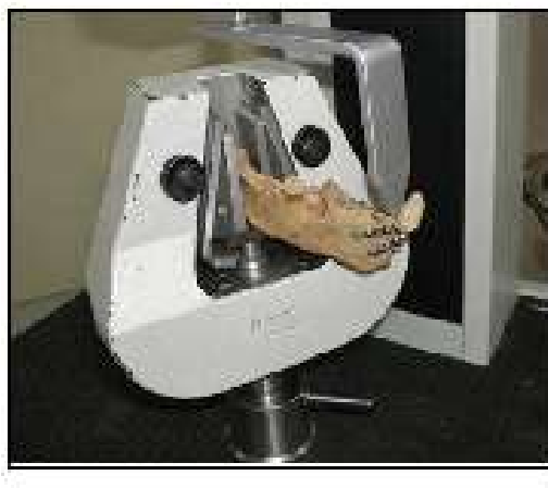
Figure Linear Load Applied in Anteroposterior Direction (Double Miniplate)
