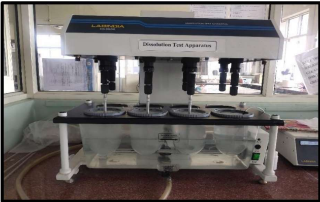
Figure 24. Dissolution test apparatus used in the source thesis.
