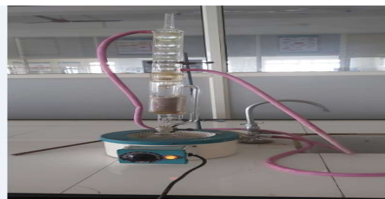
Fig. 1 Alstonia Scholaris (L.) bark extraction by soxhlet apparatus
