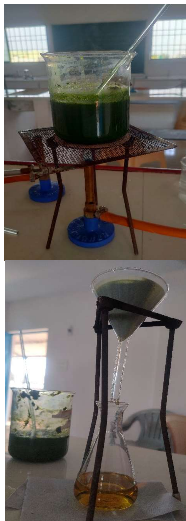
Fig. 2: (a) Homogenized garlic-leaf suspension during extract preparation; (b) filtration of the aqueous garlic-leaf extract.
