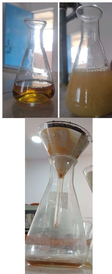
Fig. 4: (a) Reaction mixture before addition of \text{AgNO}_3 solution; (b) after addition of \text{AgNO}_3 and filtration of the synthesized AgNPs.
