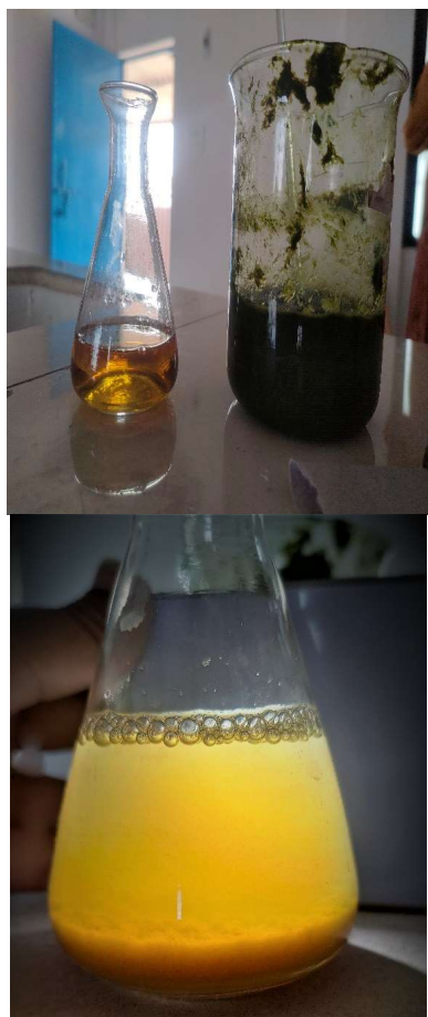
Fig. 3: (a) Clear filtrate of the garlic-leaf extract; (b) reaction mixture showing the onset of AgNP formation.
