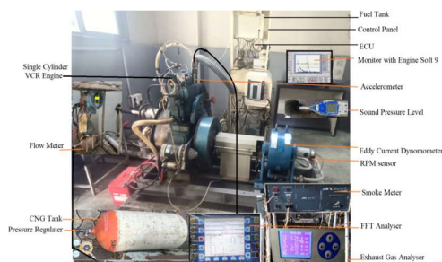
Fig 1. Experimental test rig for Dual fuel diesel engine
