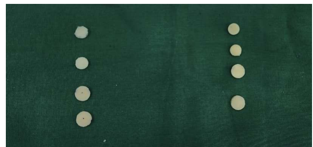
Figure 1. Standardized disc-shaped composite specimens were prepared for surface roughness and color stability evaluation.
