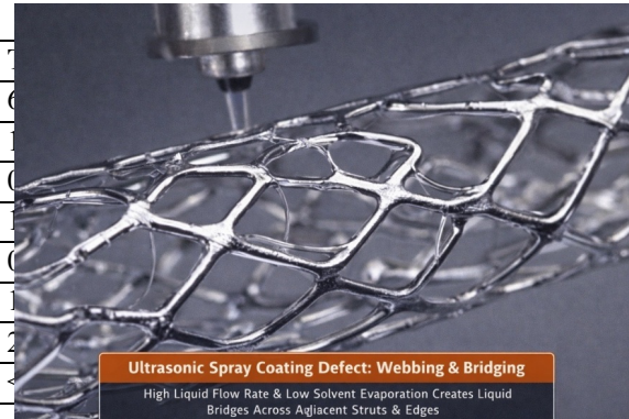
Figure 41 Coating defect - Webbing and Bridging
