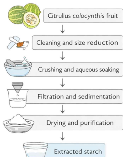
Figure 2. Schematic representation of starch extraction process from Citrullus colocynthis .
