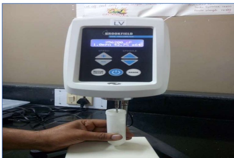
Figure.5. Representing Brookfield viscometer determining viscosity of formulation.
