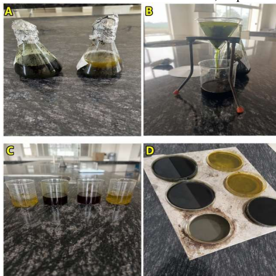
Figure 4. (A–D) Sequential steps of the maceration extraction process, from soaking of powdered leaf material through filtration and concentration of the ethanolic and petroleum ether extracts.
