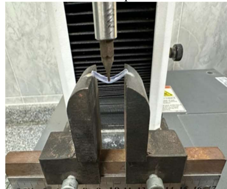
Figure (2): force applied vertically to the top of the specimen midway between two supports at cross head speed 1mm/min.
