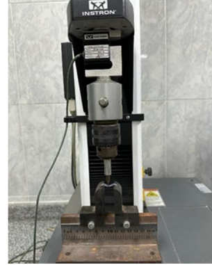
Figure (2): force applied vertically to the top of the specimen midway between two supports at cross head speed 1mm/min.
