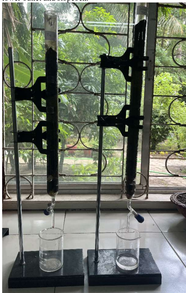
Figure 1. Laboratory Soil-Column Apparatus used for the Preliminary Alkaline Leaching Experiment. The Column was Vertically Mounted and Discharged
