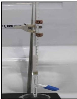
Fig. 4: DEAE-Cellulose Anion Exchange Chromatography of the sample
