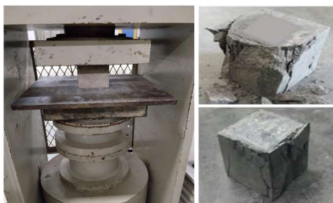
Figure 12 compressive strength of OPC-43 grade cement by adding Ce 2 Zn 4 O 7 bimetallic oxide nanoparticles
