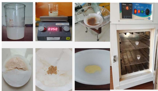
Figure 3 Photographic Representation of \text{Ce}_2\text{Zn}_4\text{O}_7 bimetallic oxide nanoparticles
