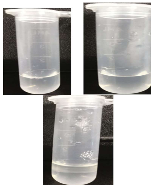
Fig. 6: Influence of three different sterilization methods on the stability of RHC-NE: (a) microporous filter; (b) UV sterilization; (c) autoclave
