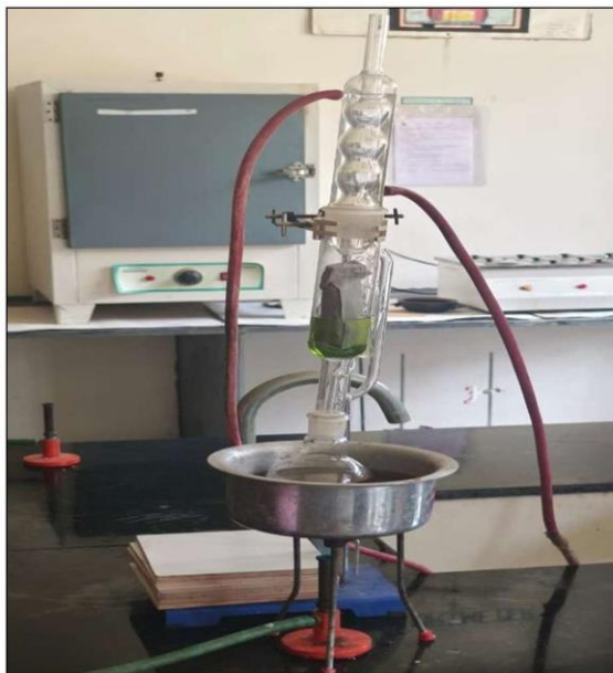
Figure 1. Soxhlet apparatus used for extraction of Salvadora persica phytoconstituents [23].
