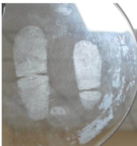
Figure 2. Fingerprint developed on a glass surface using papaya leaves powder.
