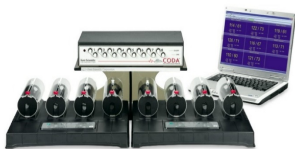
Figure 1. CODA multichannel, computerised, non-invasive blood pressure system for mice & rats
