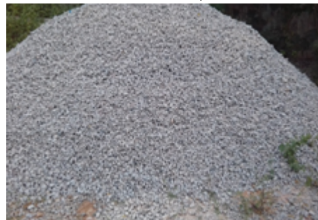
20mm and 12mm size aggregates
