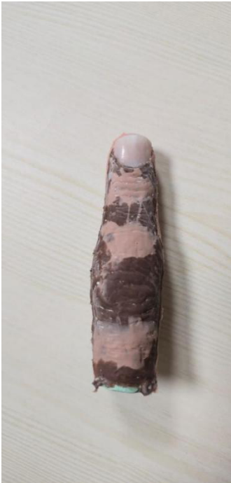
Retrieval after overnight RT cure + 1 h heat cure at 100 °C
