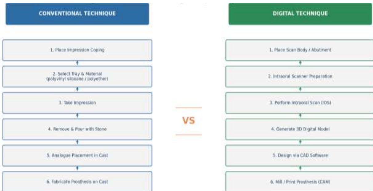
Figure 1. Workflow comparison- Conventional (left) versus digital (right) implant impression technique. The conventional path uses impression copings and elastomeric materials leading to a stone cast, while the digital path employs scan bodies and IOS technology to generate a 3D file for CAD/CAM fabrication
