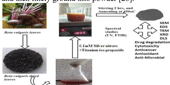
Fig 2 Scheme of green synthesis of Ag/ TiO 2 Nanoparticles
