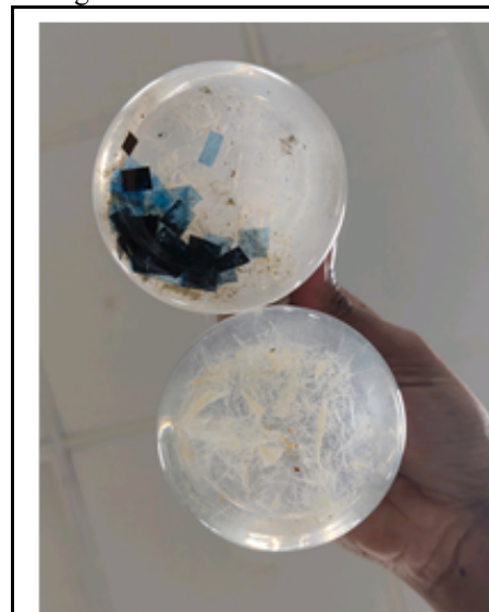
Figure: 2 X ray Film Degradation
