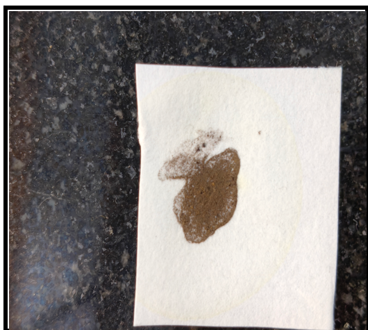
Figure: 3 Burn Test for Silver detection
