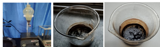
Figure 1: A graphic showing how to isolate and purify coumarin.
