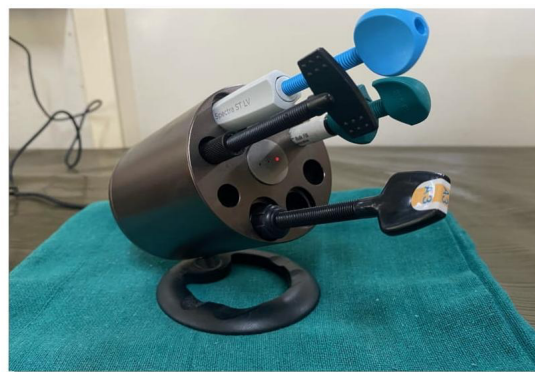
Figure 4: Composite syringes or capsules were warmed in batches using a composite heating apparatus named Endoking Nanowarm Composite Warmer at a consistent temperature of 50°C for 10 minutes
