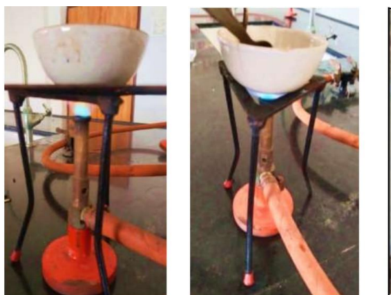
Figure 7: Determination of ash values — incineration apparatus used for total, acid-insoluble and water-soluble ash determination.
