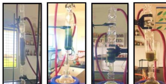
Figure 9: Soxhlet extraction set-up in the laboratory during extraction of the plant materials.
