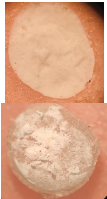
Fig no 2: cohesive and adhesive bond failure
