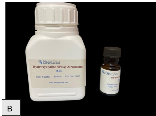
Figure 1. The materials used in the study, (A) Zirconomer-Improved Glass-ionomer, (B) Hydroxyapatite Nanoparticles added to Zirconomer-Improved Glass-ionomer.
