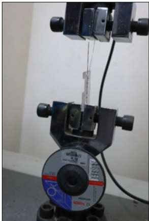
Fig 7: Testing machine with mounting template with test brackets
