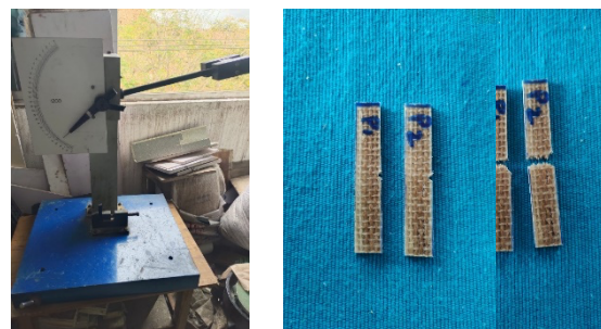
Figure. 3: Impact testing machine with samples
