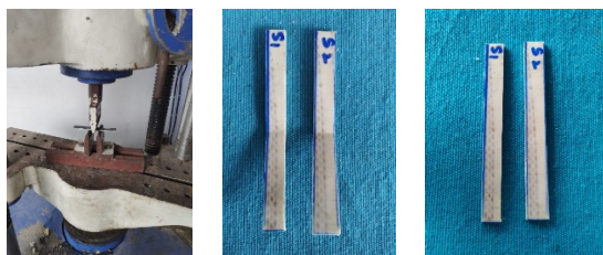
Figure. 2: Flexural testing machine with samples
