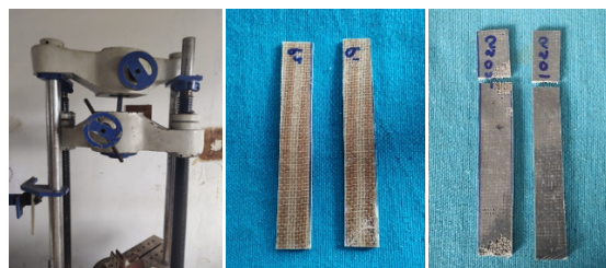
Figure. 1: Tensile Testing Machine with samples
