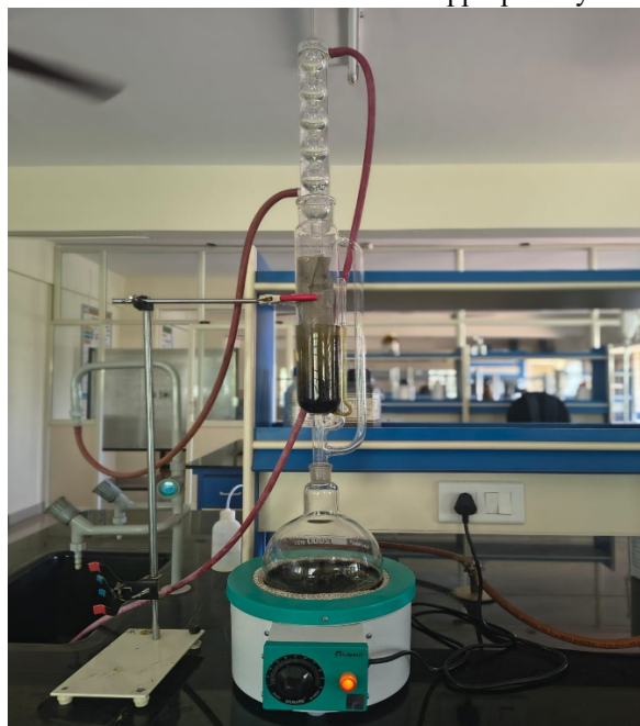
Soxhlet extraction of Ocimum tenuiflorum
