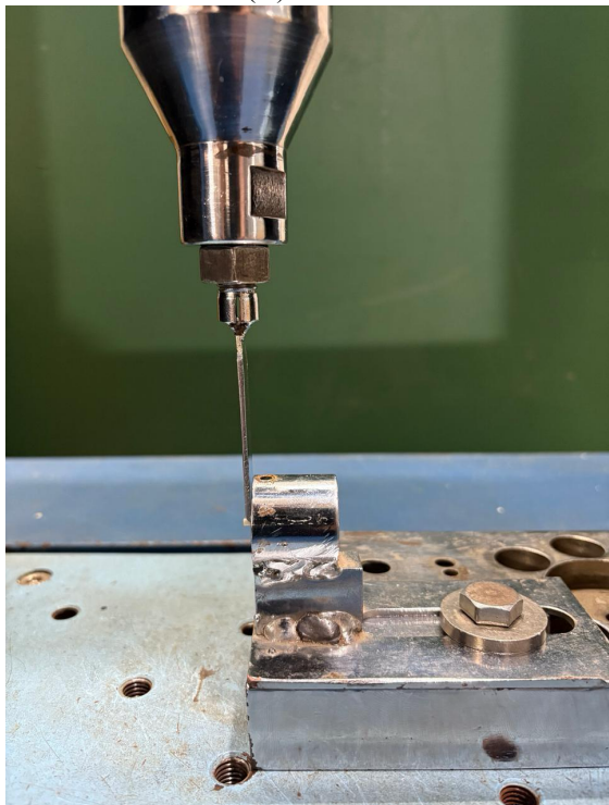
Figure 2. Microshear bond strength test set-up. The specimen is secured in the fixture of the universal testing machine and the loading blade is aligned against the repair cylinder immediately adjacent to the adhesive interface.
