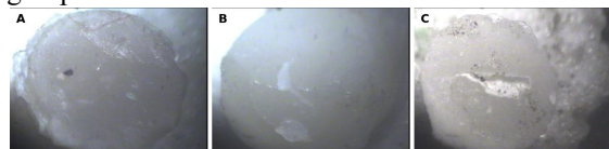
Figure 5. Representative stereomicroscopic images of debonded specimens. (A) Adhesive failure: a clean fracture along the repair interface with no composite remaining on the substrate. (B) Mixed failure: interfacial failure combined with small fragments of retained composite. (C) Cohesive failure: fracture running within the composite material, leaving a band of fractured composite on the surface.
