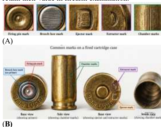
(B) Fig 1- (A) close ups of toolmarks. (B) different toolmarks of the cartridge cases in every aspect. (Xin et al., 2026)
