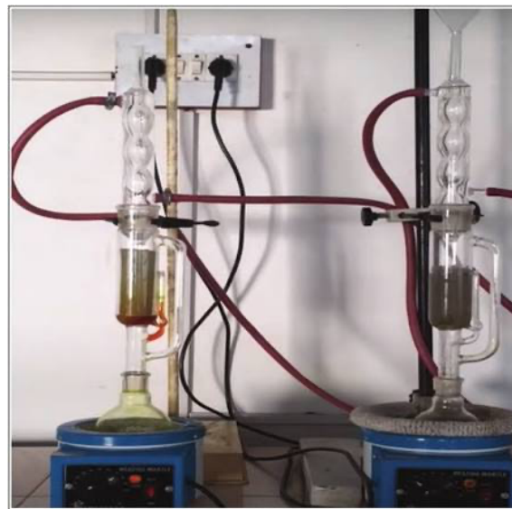
Figure 1: Soxhlet extraction of Vitis vinifera L.
