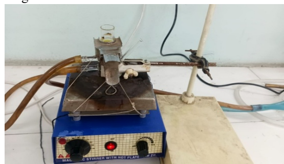
Fig: 12 Franz diffusion cell assembly utilized for monitoring the in-vitro drug release profile
