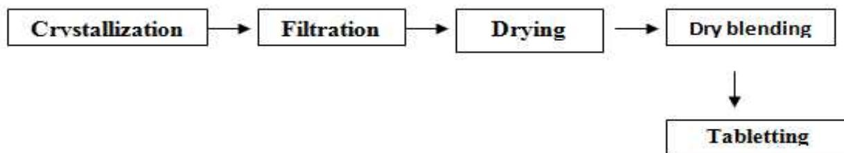
Fig 3. Spherical crystallization process
