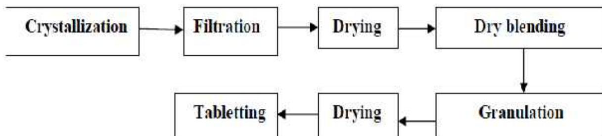
Fig 2. Traditional tablet manufacturing
