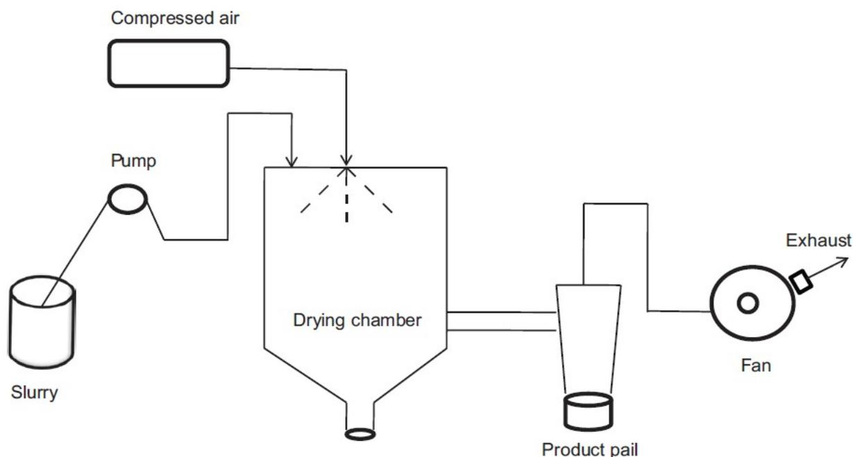
Figure 3: Spray drying method.
