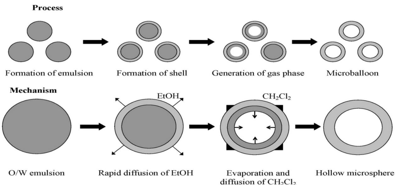
Figure 1: Solvent evaporation method.
